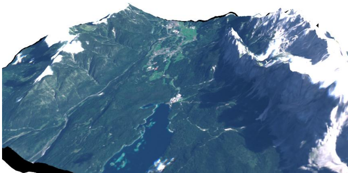
Figure 5 - WCPS query with result visualized through terrain draping in WebGL
