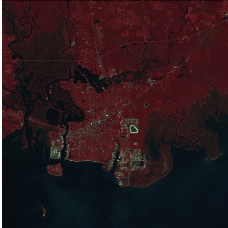
Figure 20: False color image constructed from the near IR, red and green bands.
