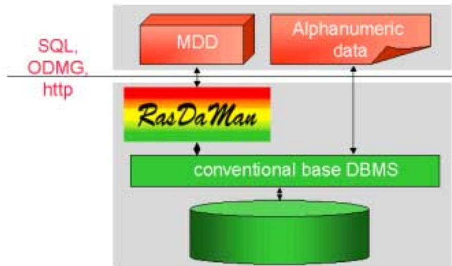
**Fig. 3.** Embedding of RasDaMan into overall data management
